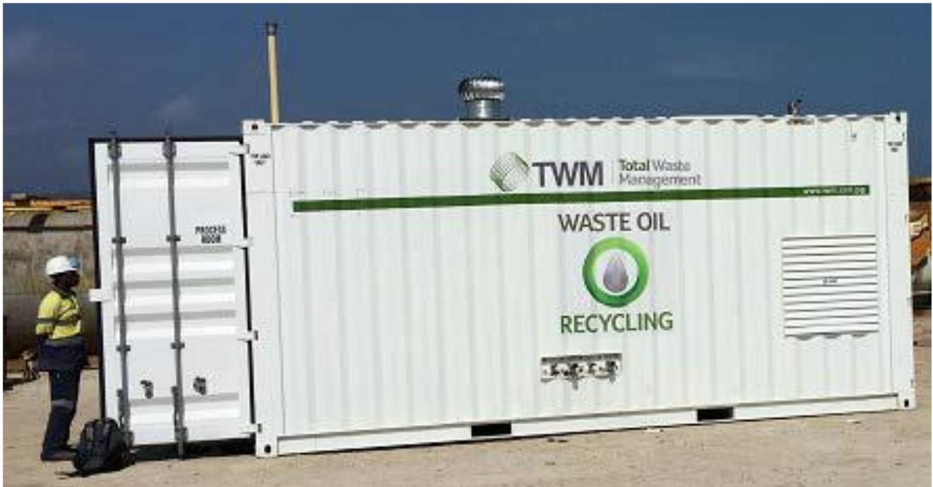
Figure 8 Containerised used oil processing and fuel blending unit (PNG)<sup>35</sup>
